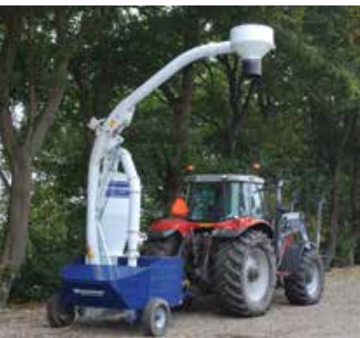
Loading equipment on SupraVac 2000 ready for loading grain onto lorry.
